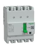
Circuit breaker, GoPact MCCB 125, 4 poles, 15kA at 415VAC, 100A rating, TMD trip unit, adjustable thermal protection
