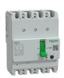
Circuit breaker, GoPact MCCB 125, 4 poles, 15kA at 415VAC, 20A rating, TMD trip unit, adjustable thermal protection
