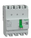
Circuit breaker, GoPact MCCB 125, 4 poles, 15kA at 415VAC, 20A rating, TMD trip unit, fixed thermal protection
