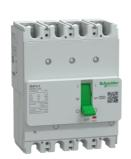
Circuit breaker, GoPact MCCB 125, 4 poles, 15kA at 415VAC, 32A rating, TMD trip unit, fixed thermal protection
