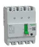
Circuit breaker, GoPact MCCB 125, 4 poles, 30kA at 415VAC, 20A rating, TMD trip unit, adjustable thermal protection
