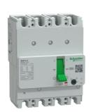
Circuit breaker, GoPact MCCB 125, 4 poles, 10kA at 415VAC, 125A rating, TMD trip unit, adjustable thermal protection
