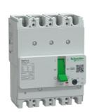
Circuit breaker, GoPact MCCB 125, 4 poles, 10kA at 415VAC, 25A rating, TMD trip unit, adjustable thermal protection
