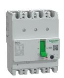
Circuit breaker, GoPact MCCB 125, 4 poles, 10kA at 415VAC, 40A rating, TMD trip unit, adjustable thermal protection
