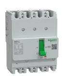
Circuit breaker, GoPact MCCB 125, 4 poles, 10kA at 415VAC, 32A rating, TMD trip unit, fixed thermal protection
